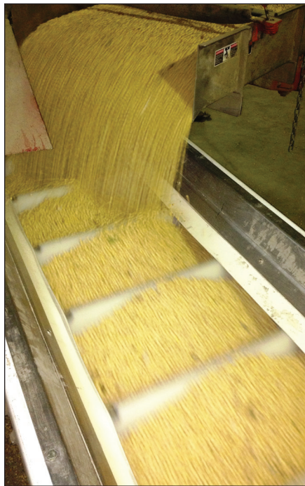
A vibratory conveyor moving soybean seed into an Anex Mfg. cup elevator with a low vertical drop.
