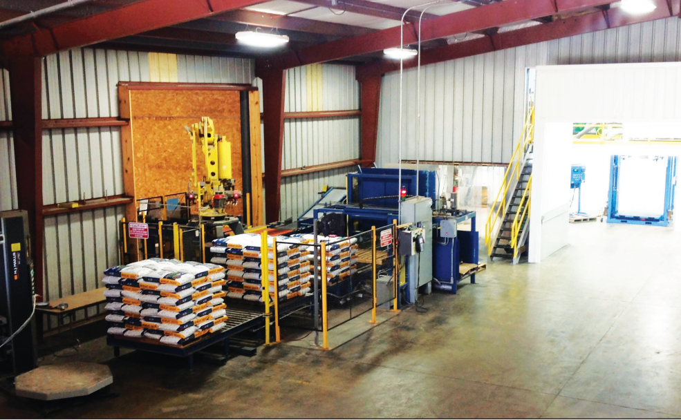
The existing pallet feeder and robotic palletizer have sufficient capacity to be retained and used in the expanded facility.
